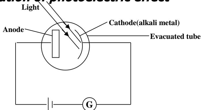
When light falls on a metal cathode, a galvanometer shows a deflection, indicating flow of current. However when the plates are covered, more current flows. Energy of the incident light is absorbed by the electrons and instantly an electron jumps out. Such ejected electrons are called photoelectrons.
