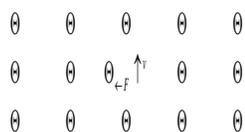
The magnetic force on the electron is  $F = Bev$  and using Flemings left hand rule it is at right angles to both  $v$  and  $B$ .
