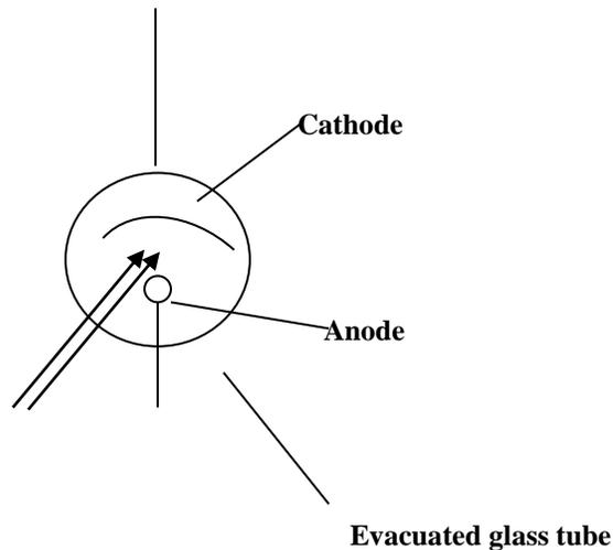
The cathode is curved metal plate having an emissive surface facing the anode. When electromagnetic radiation fall on the cathode, photoelectrons are emitted and are attracted to the anode if it is a suitable positive potential. A current of few microamperes flows and increases with the intensity of the incident radiation.
