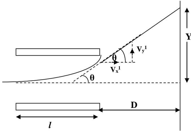
The time taken by the electron to move through the plates  $t_1 = \frac{l}{u_0}$
