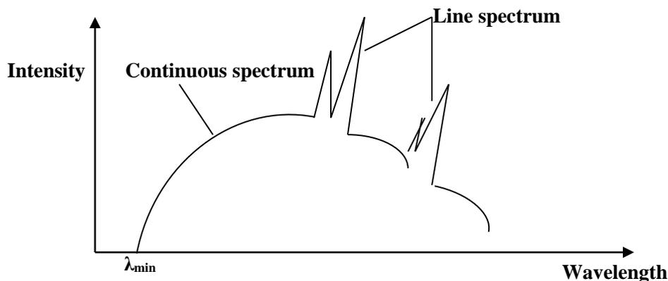
When an electron loses all its energy in a single collision with an atom of the target, a most energetic x-ray photon is given off. The kinetic energy of the electrons equal to  $eV$ , where  $V$  is the accelerating voltage between a filament and the anode. It is converted into electromagnetic radiation of
