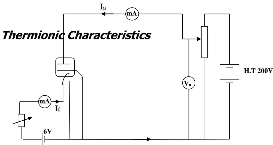
Keeping the filament current  $I_f$  constant, the p.d  $V_a$  between the cathode and the anode is varied. The corresponding anode current  $I_a$  is measured. A graph of  $I_a$  against  $V_a$  constitutes the anode – current anode voltage characteristics. By setting the filament current to other constant values, the corresponding  $I_a$ - $V_a$  characteristics can be obtained. These features can be shown below
