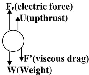
At terminal velocity,  $v_1$
