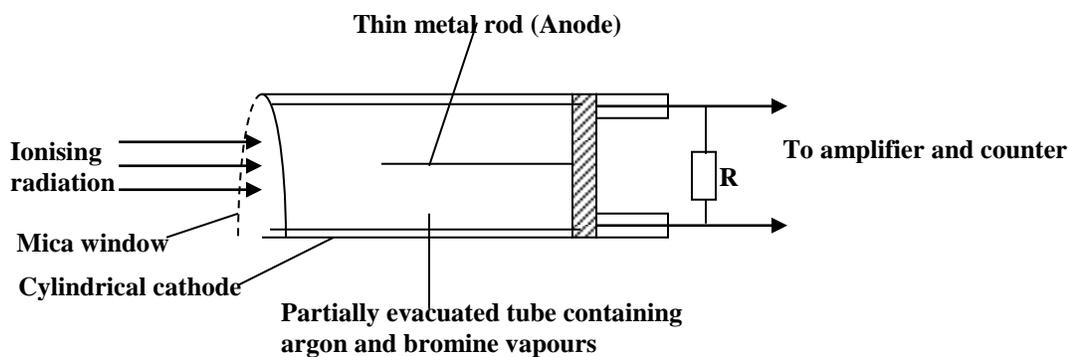
When the radiation enters the tube, it causes ionisation of the gas atoms. The electrons produced are accelerated to such a high energy that they also cause more ion pairs by repeated collisions. When the electrons reach the anode, the pulse is produced which is amplified and detected by a rate
