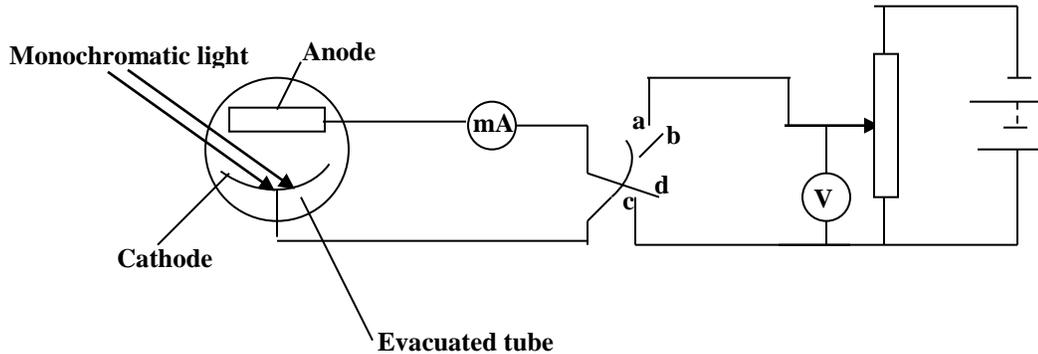
With a connected to b and c to d, the photocurrent  $I$  is measured for increasing values of  $V$ . A graph of  $I$  against  $V$  is plotted and has the form shown below;
