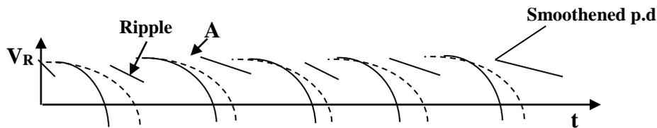
At points such as A, the p.d across the load has just reached its maximum value. If the capacitor was not present, the p.d would start to fall to zero along the broken curve. However, as soon as the p.d across the load starts to fall, it becomes less than that across the capacitor and the capacitor starts to discharge through the load.
