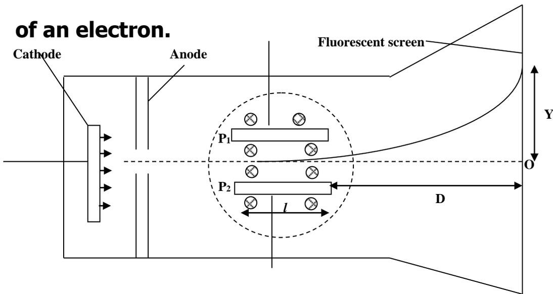
Electron emitted by the heated cathode is accelerated to the anode. In the absence of the electric and magnetic fields, the cathode rays strike the fluorescent screen at O. The p.d is then applied between plate's P<sub>1</sub> and P<sub>2</sub>. The deflection Y of the cathode rays is measured. A magnetic field is then applied to the plane of the figure by passing current through a pair of circular coil one on each side of the glass tube.
