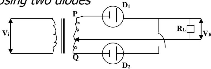
When P is at negative potential relative to Q, diode  $D_1$  conducts whereas  $D_2$  doesn't.
