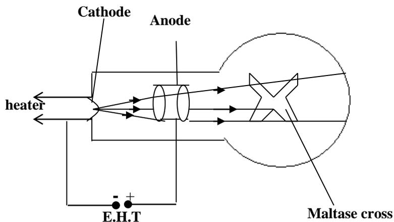
If an opaque object (Maltse cross) is placed in the path of the cathode rays, a sharp shadow of the Maltse cross is cast on the screen.
