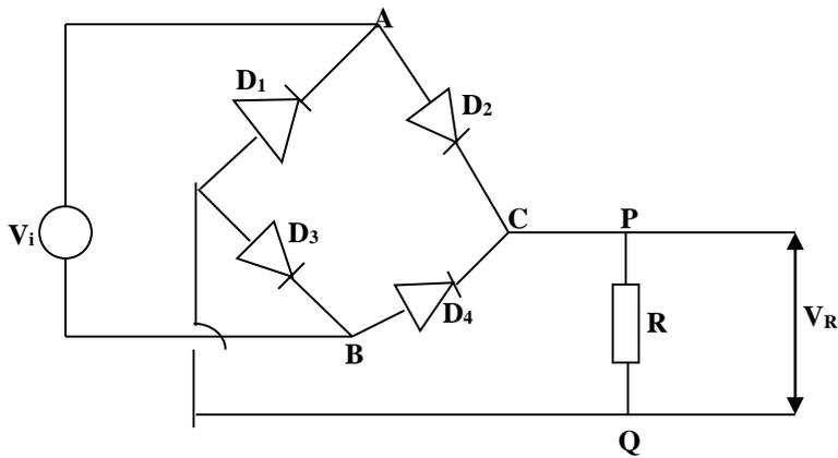
During the half cycles when A is at positive potential relative to B, diodes  $D_2$  and  $D_3$  are forward biased hence they conduct and current flows through the resistor R in the direction P to Q. Diodes  $D_1$  and  $D_4$  are reverse biased and they do not conduct.
