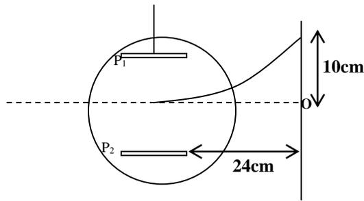
In the figure,  $p_1$  and  $p_2$  are metal plates each of length 2cm and separated by 0.5cm in a uniform magnetic field of flux density  $4.7 \times 10^{-3}T$ .
