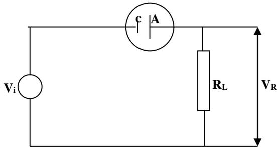
During the half cycles when A is positive relative to C the diode conducts and a p.d  $V_R$  appears across the load  $R_L$ . During the half cycles when A is at a negative potential relative to C, the diode does not conduct and no p.d appears across  $R_L$ . The a.c is half-wave rectified.
