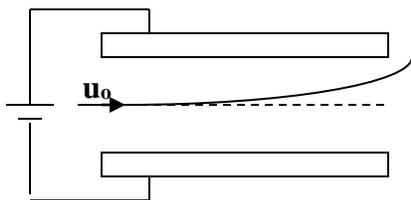
Consider an electron of speed  $u_0$  entering mid way between metal plates  $P_1$  and  $P_2$  separated by a distance  $d$  and across which a pd  $V$  is applied. The electric force has no component in the horizontal direction. Hence, the horizontal component of the electron velocity stays constant at the values  $u_0$ . The vertical component of the electrons velocity at a time  $t$ , after the electron has entered the region of electric field is  $V_y = a_y t$
