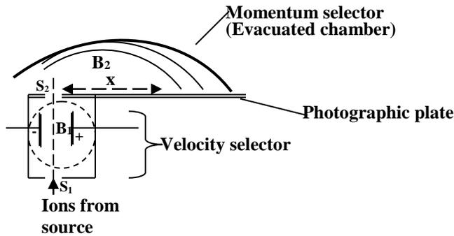
Ions from the source enter the velocity selector through collimating slit  $s_1$ . The ions enter the velocity selector and only ions with velocity  $v = \frac{E}{B_1}$  pass through undeflected.  $E$  is the electric field intensity of electric field in the momentum selector,  $B_1$  is the magnetic flux density of the magnetic field in the velocity selector.
