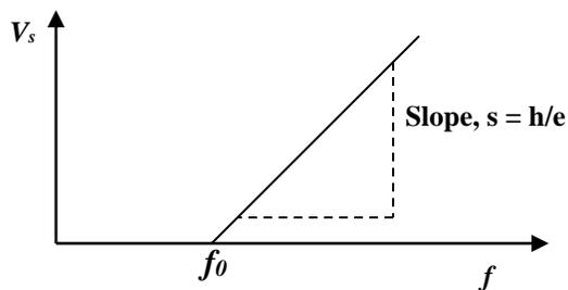
The slope of the graph,  $s = h/e$ , where  $e$  is the electronic charge
