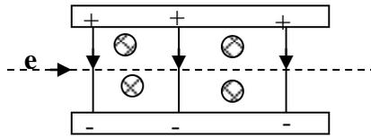
Consider an electron projected with a speed  $v$  at right angles to both electric intensity  $E$  and magnetic flux density  $B$ .
