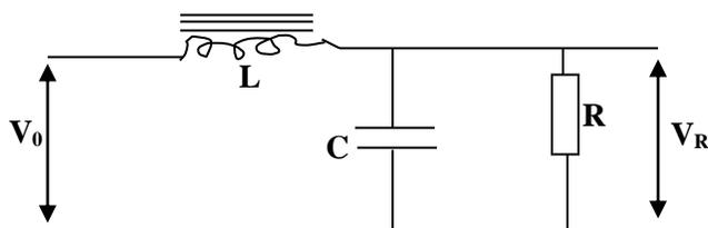
The back emf induced in the inductor by the fluctuating voltage opposes the voltage fluctuations. The capacitor acts as a reservoir to steady the remaining voltage fluctuations.
