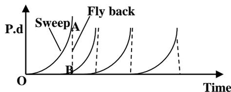
The time taken for p.d to fall from A to B known as the fly back time, is extremely small compared to the time taken to rise from O to A. Hence the time taken by return of the electron beam to the original position at the other end of the screen is small.
